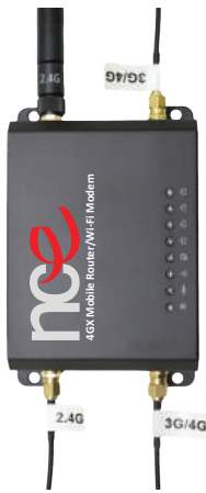
External Antenna Installation
